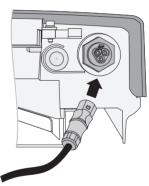
☑ The AC cable is connected to the inverter.
