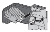
6. Insert the fan plug (A) into the jack. The fan plug snaps audibly into place.
