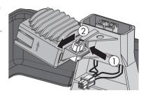
4. Clean the enclosure and the fan with a soft brush, a paint brush, or a damp cloth.
