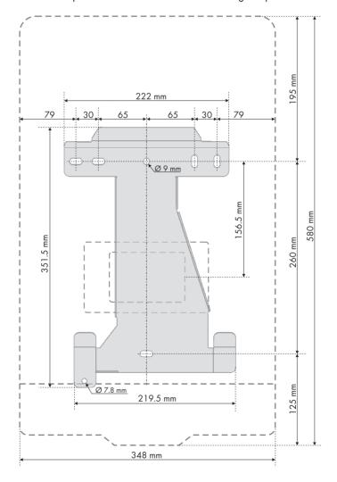
Attach the wall mounting bracket to the wall using appropriate screws (diameter min. 6 mm, max 8 mm) and washers (outer diameter min. 12 mm, max. 24 mm).
