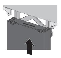
Check that the Quick Module is correctly seated.
