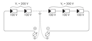
In this case, the ground fault is between the second and third PV modules.
