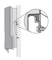
6. Use the connection elements (see item "M" in the scope of delivery on page 13) provided to fix the inverter and prevent it from being lifted out of place. To do this, push the connection elements through the plastic flap on the bottom of the inverter and into the wall mounting bracket.
