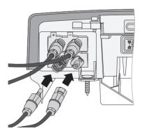
Plug in the Electronic Solar Switch. If an RS485
