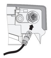
Check the DC connectors for correct polarity and connect them.
