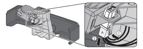
Push the latch on the retainer of the Electronic Solar Switch downwards (1) and at the same time remove the fan enclosure together with the fan (2).
